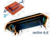
1 barrier prevents water ingress 2 barriers block wind driven rain 3 water drains away down slope
